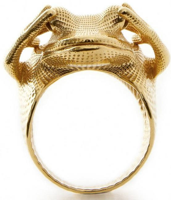
Figure 4: A gold plated brass 3D print ring [10].
