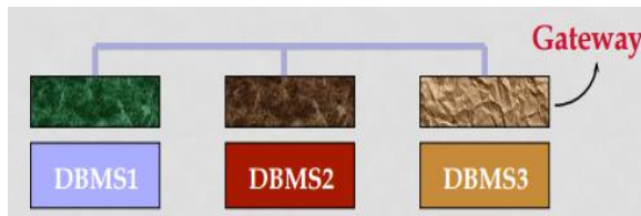
Figure 2: Heterogeneous DBs Communicate Through Gateway Interfaces
