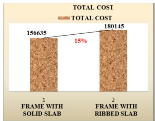
Figure 7: Result of Comparison of Total Cost between Frame with Solid and Ribbed Slab
