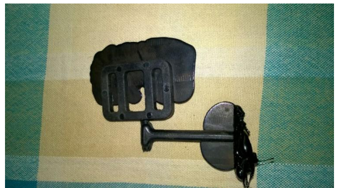
Picture 3.1: Mold Flash Defect
