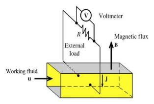
The set of equations which describe MHD are a combination of the Navier-Stokes equations of fluid dynamics and Maxwell's equations of electromagnetism.
