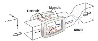
Since the plasma temperature is typically over 2000 °C, the duct containing the plasma must be constructed from non-conducting materials capable of withstanding this high temperature. The electrodes must of course be conducting as well as heat resistant.
