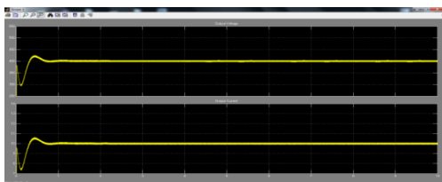
Fig.14 Output voltage and output current of PFC mode controlled converter
