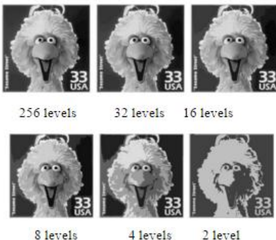
Figure 9: Quantizing a Gray-Level Image
